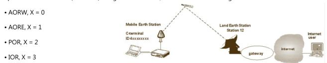
Note that the LESs 02 and 12 are operated independently from each other, therefore in order to use both LESs at any time, you must register for service on both. Once registered on a specific LES (02 or 12), email users can send messages to any Inmarsat-C terminal. The basic format for sending messages is as follows:
