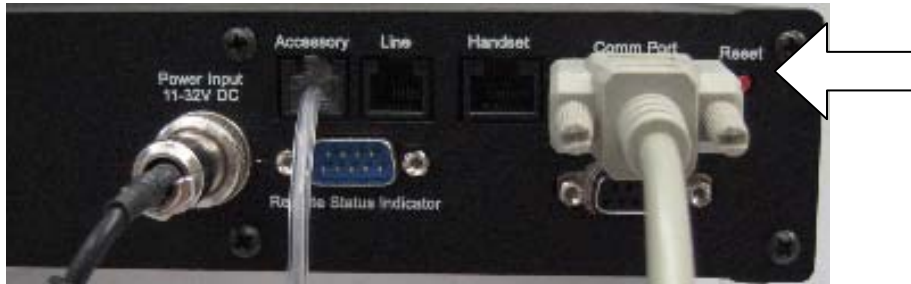
Figure: Serial cable connected to Comm Port
