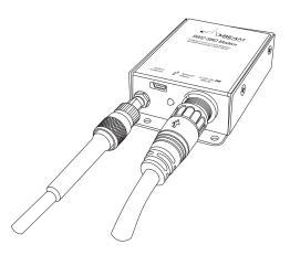
The default baud rate is 19200 8N1 with hardware hand-shaking (CTS/RTS). The 9602 SBD MODEM does not have an autobaud facility. The baud rate can be set via the AT+IPR=n where n is one of the following.
