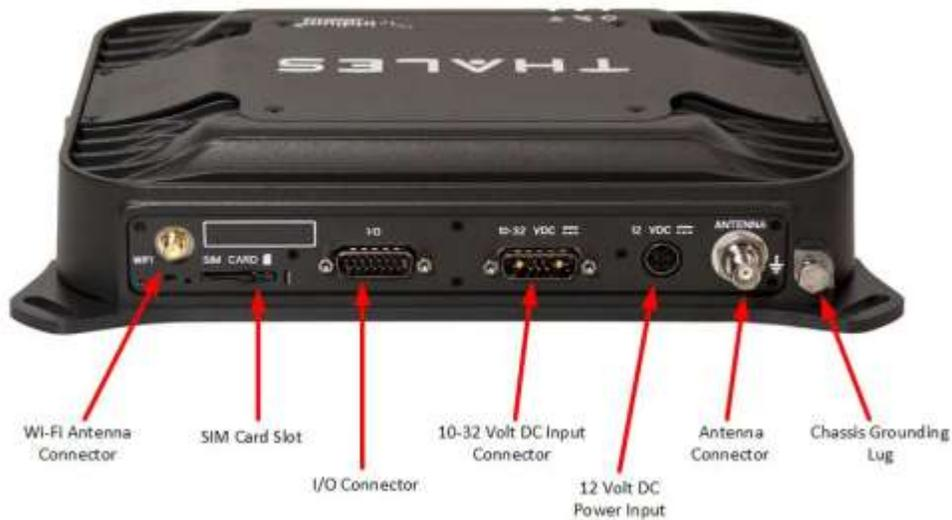
*Figure 2-7 Terminal Unit (TU) Back Panel Detail*
