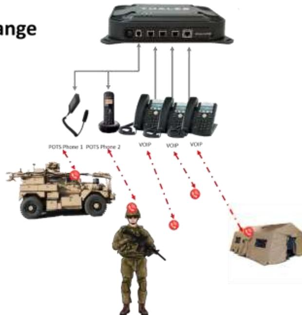
Figure 2-2 Local Communications via PBX Functionality
