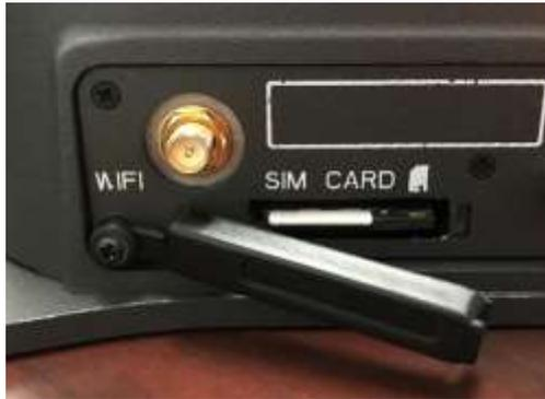
*Figure 3-3 SIM Card with Cover Opened*
