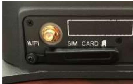
Figure 3-5 Secure the SIM Card Cover
