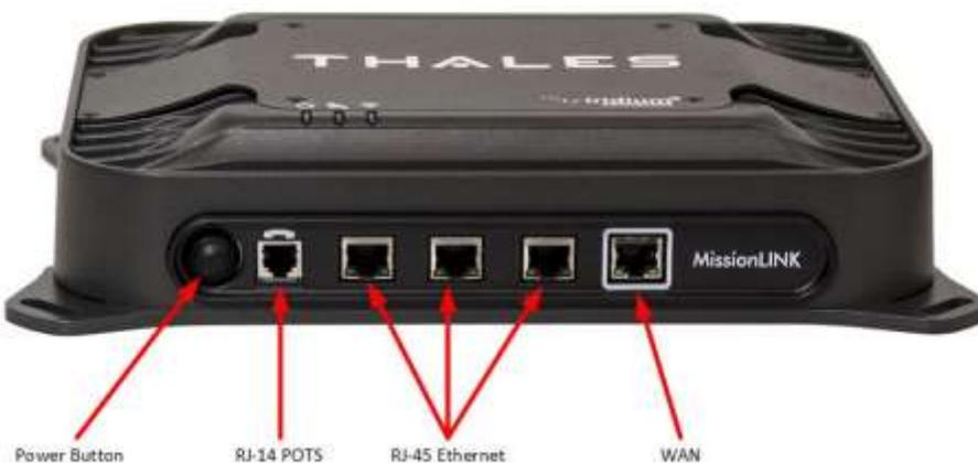
*Figure 3-1 Terminal Unit (TU) Front Panel Detail*
