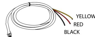
The DC power cable has three wires, RED, BLACK and YELLOW. The RED and BLACK wires are used for the power connection while the YELLOW wire can be connected to a switch.
