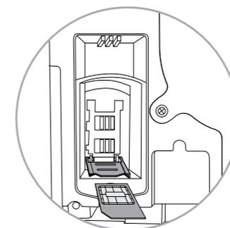
5. Gently insert the SIM card into the tray slots making sure that the golden contacts are facing downwards.
