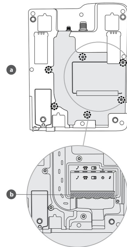
3. The USB rubber cap is required to ensure ingress protection.
