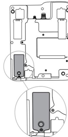
3. The SIM connector is shown highlighted below. Slide the tray guide into the open position with your finger or thumb.
