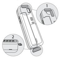
To dock the handset, align the IsatPhone Pro with the phone tray and slide the handset down until it seats flush to the bottom of the tray. Swing the phone down into the cradle by applying pressure to the top of the handset. An audible 'click' is heard when the phone is in the docked position.
