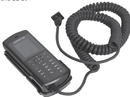
The Primary Handset's RJ45 connector is plugged into the BDU's primary handset port and it is powered directly from the BDU. For information on how to use the handset, see Chapter 3, Using the Primary Handset.
