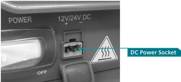
2. Connect the power cable to the vessel's DC power supply. More information of power supply input, please refer to Chapter 7 of this user guide.
