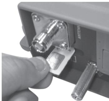
5. Use your finger to push the SIM card gently until it is being clicked and locked in place. Any screwdriver can be helped to push the SIM card if the SIM card cannot be inserted properly.
