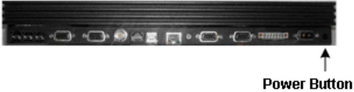
Press and hold the power button for a few seconds or until the green LED on the front of the terminal lights up.
