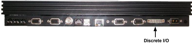
The BDU also has a discrete I/O interface, containing 4 configurable input/output.
