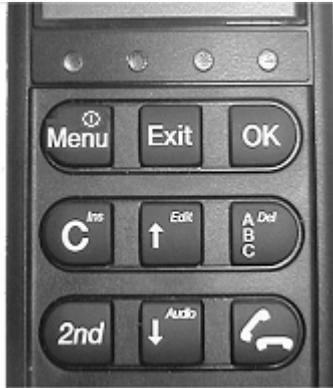
The Function keys, as shown above, enable the user to enter the menu system of the BDU and change various settings.
