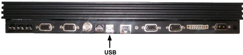
USB - Universal Serial Bus - is an interface that allows a single universal plug to connect PCs. USB replaces the different serial and parallel PC connections with one standard plug-and-play port. Please note that the USB interface only supports the 64 kbit/s UDI service at present time.
