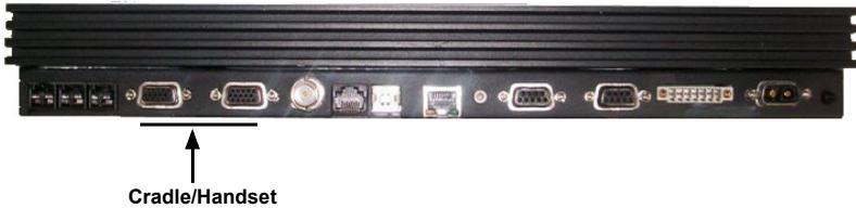
The BDU has two 4 wire handset ports with RS-485 data control.
