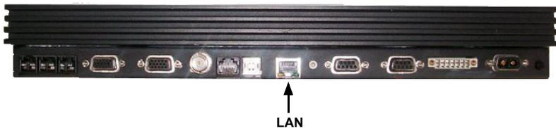
The Ethernet interface is a RJ45 connector. It can be used for the MPDS service. Connect a computer through a switch or hub or connect directly using a crossover cable.
