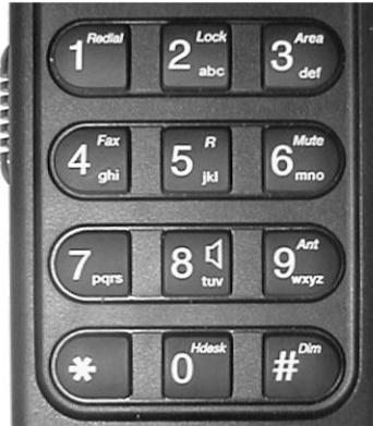
The keypad can be in normal (numeric) mode or alpha mode. Normal mode is used to enter digits (phone numbers) whereas alpha mode is used to enter letters (names in the phone book). The key is used to switch between the two modes and the display indicates if the keypad is in alpha mode.
