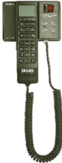
The cradle has a distress button, a stop button and three LEDs. The distress button, which is protected by plastic glass, is used to initiate a distress call. The stop button can be used to abort a distress call. The three LEDs indicate power, distress test and priority calls. For a detailed description of the cradle see the section *Distress Cradle* on page 33.
