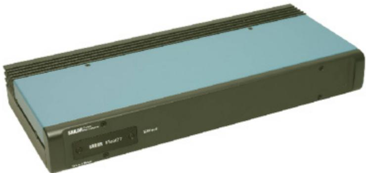
All connectors for external equipment are placed on the rear of the BDU. On the front a configuration module is attached. This module stores all system configuration data. It contains all necessary data to recover the system after a replacement of the BDU.
