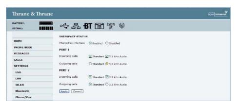
Set the Phone/Fax port to which the Omnisec 222 is connected to 3.1 kHz Audio for Outgoing calls.
