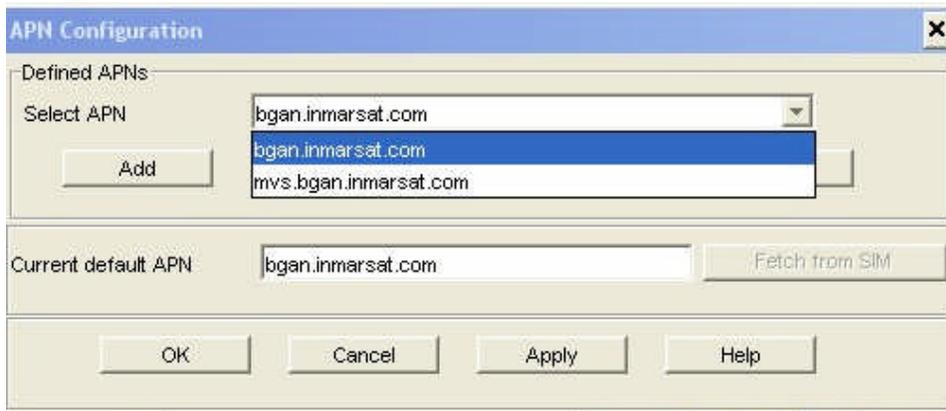
Check the displayed APN in the **Select APN** field. If it is not correct, select the required APN (for example, **mvs.bgan.inmarsat.com**) from the drop-down list and click on the “**Edit**” button.
