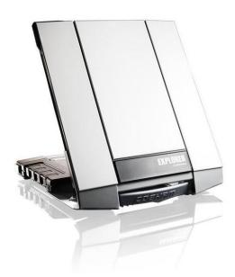
The new **EXPLORER 710** is the world's smallest Class 1 BGAN terminal and the first to take advantage of Inmarsat's new service, BGAN HDR (High Data Rate), providing on-demand streaming. The EXPLORER 710 will deliver high-speed, ultraportable satellite streaming at rates of **up to 800kbps** out of the box for broadcasting and other IP-based industry applications.
